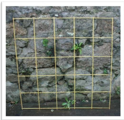
*One metre square planning frame made from steel reinforcing mesh*
